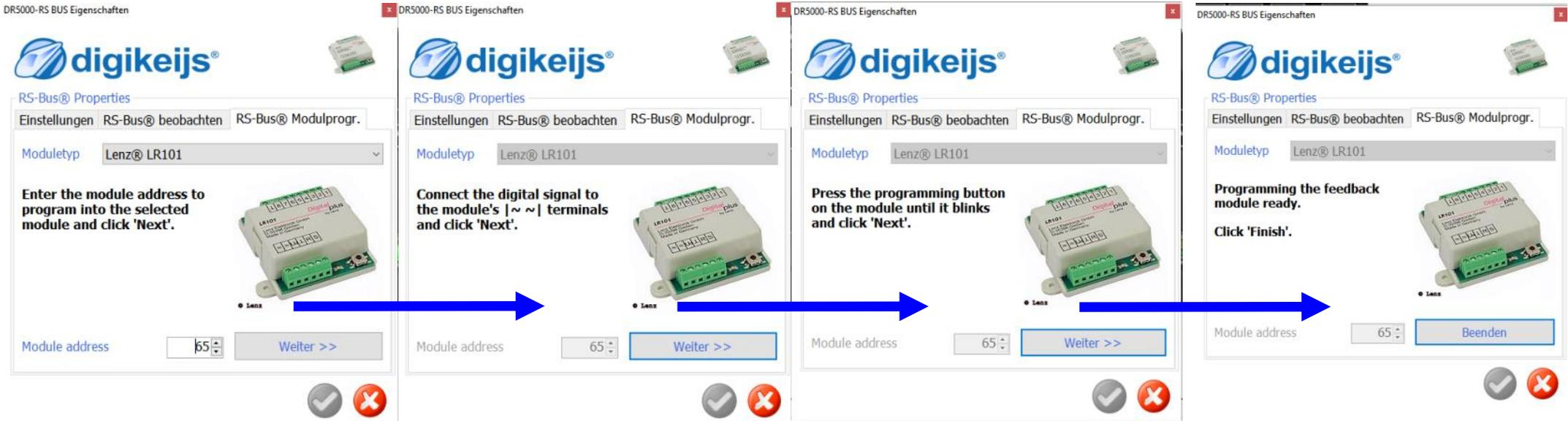
The image displays four sequential screenshots of the digikeijs software interface, illustrating the step-by-step configuration process for an RS-Bus module. Each screenshot shows the 'DR5000-RS BUS Eigenschaften' window with the 'RS-Bus® Properties' tab selected. The 'Moduletyp' is set to 'Lenz® LR101'. The 'Module address' is set to 65. The interface includes a 'Weiter >>' button and a 'Beenden' button. The steps are as follows:
