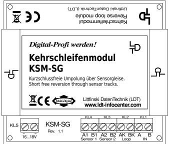
The **input A** and **B** of the **reverse-loop module KSM-SG** will receive the digital current from the command station or from a booster from the ring-conductor "driving". It is important that the **reverse-loop** will be **complete inside one booster area** and not between two rail sections which get the supply from two different boosters.
